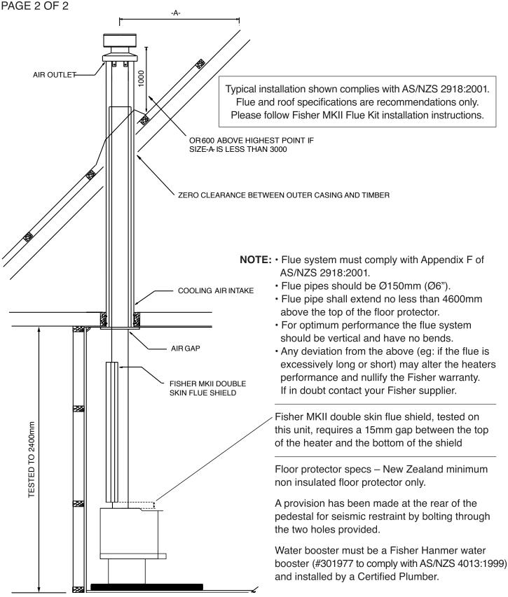
IF INSTALLED IN ACCORDANCE WITH THESE SPECIFICATIONS THE HEATER COMPLIES WITH AS/NZS 2918:2001 including Appendix F.
