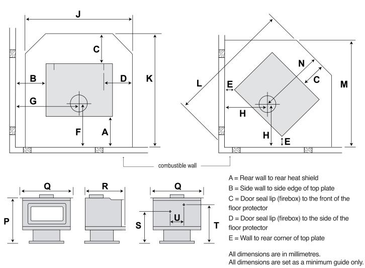
Minimum clearance requirements to combustible with 1200mm Fisher MKII double skin flue shield
