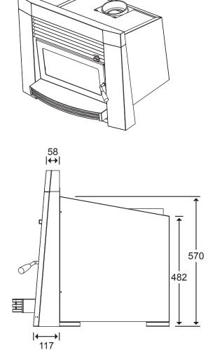
MEASUREMENTS EXCLUDE INSULATING BLANKET All dimensions are in millimetres.
