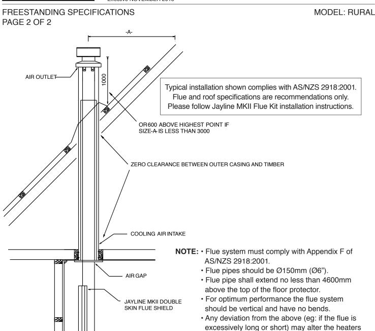
Jayline MKII double skin flue shield, tested on this unit, requires a 20mm gap between the top of the heater and the bottom of the shield
